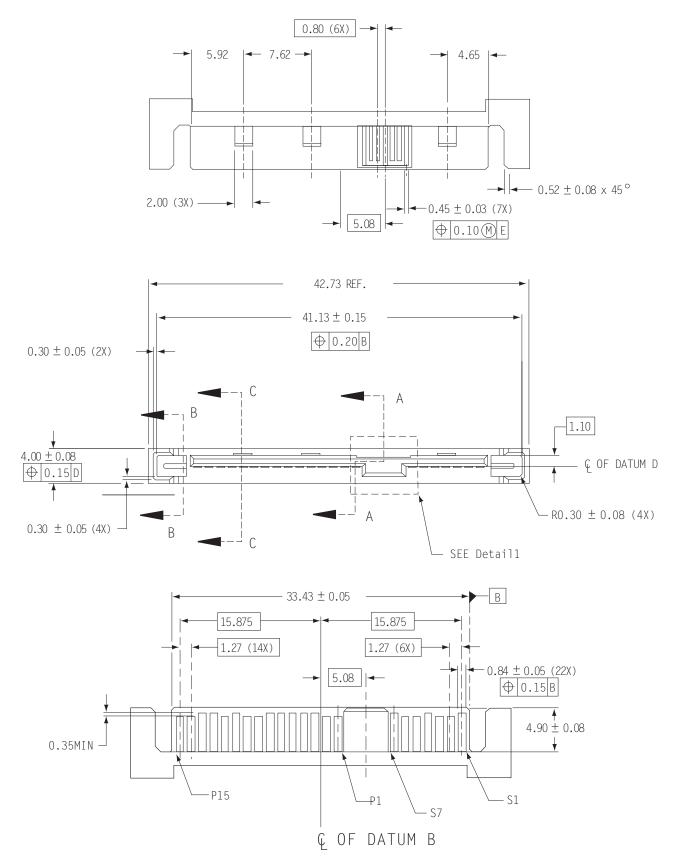
Figure 14. SAS device plug dimensions
